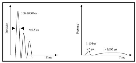
**Figure 1.**Physical characteristics of extracorporeal shock-wave therapy (ESWT) (left) and radial shock-wave therapy (RSWT) (right).
